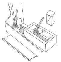
Replace the ash trap doors and firepot. Slide the ash pan trap door forward.
